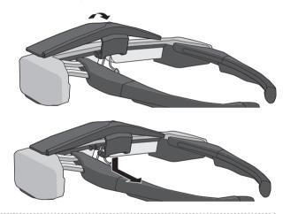
If the shade is pushed or pulled with too much force, the shade and the lens could be damaged. Do not use too much force on the shade.
