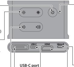
Connects to external devices that support USB Type-C. You can input video signals and supply power from the connected device. You can also output camera data and sensor data from the head-set to the connected device.
